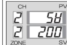
Pressing CH key to change Num. "1" into "2" in channel number, Num. "1" is changed into Num. "2"
