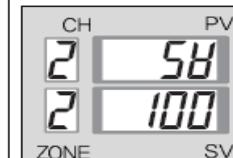
Pressing key to change 200 into 100 in SV of Num. "2" three times. It is flickered in 100 by doing V key once. Pressing key once, 200 is changed into 100 and it is flickered in that time. And then Flickering operation is stopped & registered by doing ENT key.
