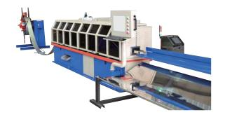
The PROFORMER steel framing system is a modern method of rapid, quality construction using light gauge steel. The PROFORMER steel framing machines make all punching and fixing holes by accurate computer control. This allows Frames or Trusses to be manufactured with high precision and enable the frame to be self locating.
