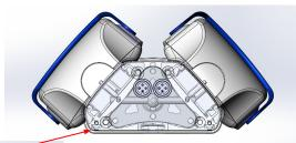
This part will be screw with the active end of gas strut, and I have thought to take a 8mm rod through this part and outer extrusion then the whole outer extrusion assembly will be lifted
