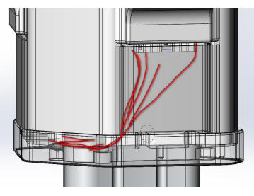
These red line is for showing how the wire to through to the clamp head to slave,
