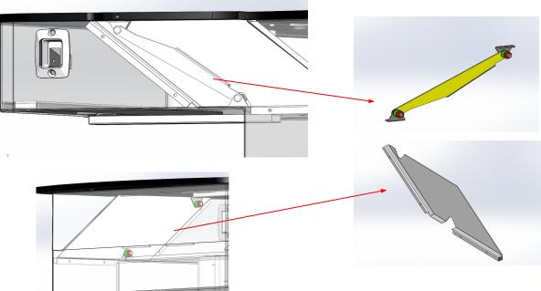
• This medicine cart will be seen the whole inner area, so I have thought to take the bowden wire to as the way to active the gas strut, and that could be no need to design the lever system to transmit the force, and make the inner side as clean as possible. as the below picture shown
