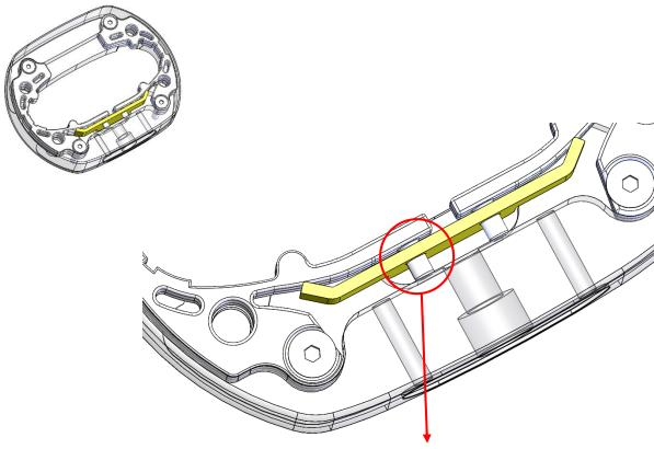
• The round pin extrude from Nylon bearing, which is hang on the sheet metal to insure sheet metal on the right position.
