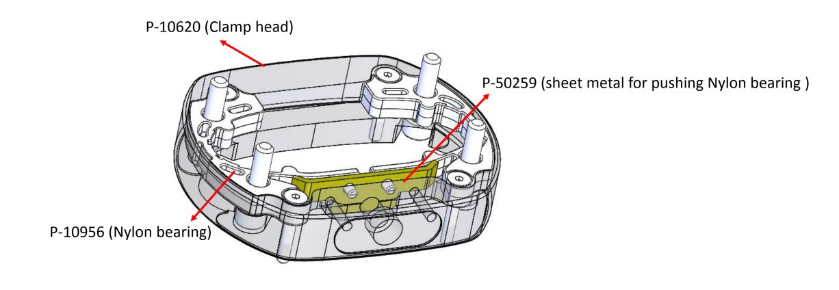
• According to the previous discussion on Wrike in 09 Mar, if we want to thicken the clamp head to 28mm, we need to tool a new core mold for it so we roll-back to the original design clamp head(18mm).
